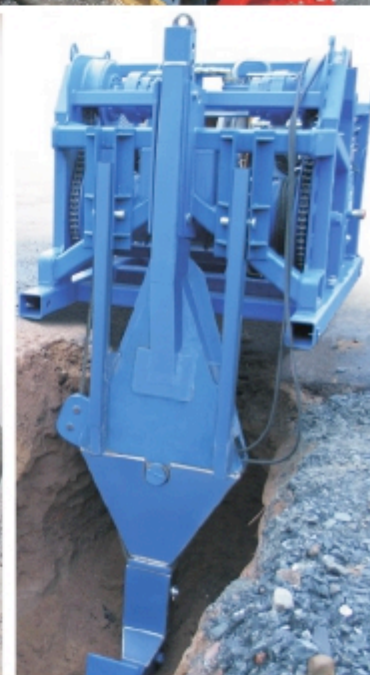
The 30 ton winch unit delivers enough power for even the heaviest pulling jobs.
